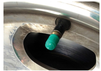
Tires with green valve stem caps are filled with nitrogen, instead of compressed air.
